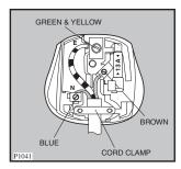
The wire coloured green and yellow must be connected to the terminal marked with the letter «E» or by the earth symbol = or coloured green and yellow.
